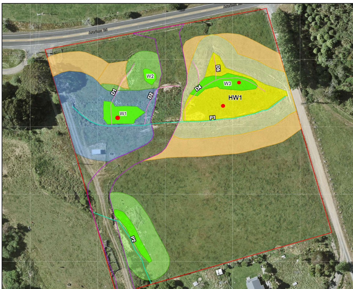
Figure 9: Indicative locations of shallow groundwater piezometers (red dots) – northern end of site.
